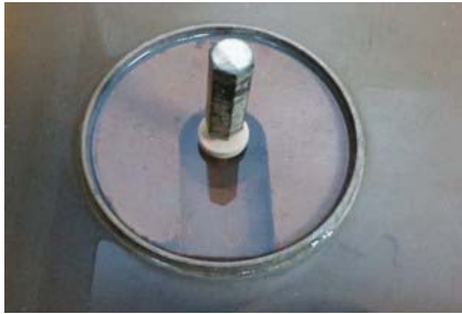
Figure 2. Soil sample during soak for CBR test
