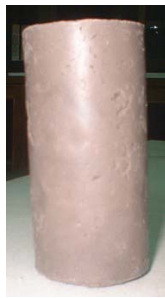
Figure 1. Stabilized soil sample for UCS test
