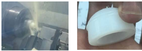
Figure 18. Manufacturing process and Test specimen of liner
