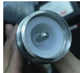
Figure 22. The break of liner after Experiment
