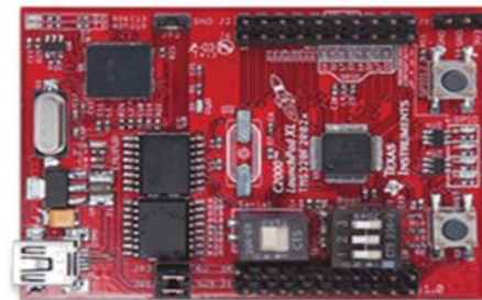
Fig. 1. Experiment kit TMS320F28027 (C2000 LaunchPad XL)
