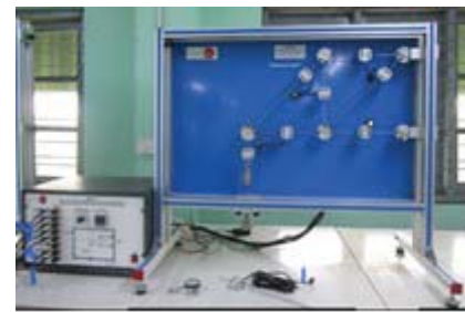
Figure 6. Unit for studying forces in an overdeterminate truss (MFCS-2 unit).
