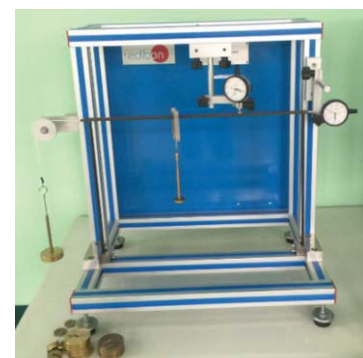
Figure 8. Deflection measurement of portal frame unit (MPO unit).
