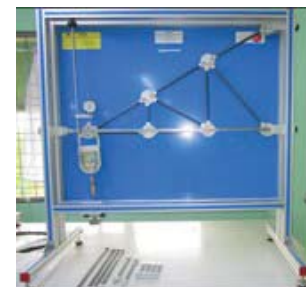
Figure 7. Unit for studying deformation of truss (MFCS-3 unit).
